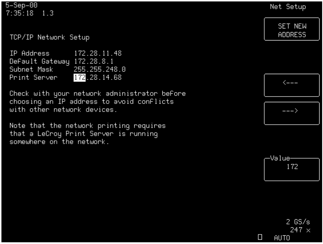
Figure 6-2. Screen used to set up network printer
